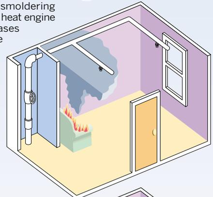
**2** As soon as the trigger mechanism is heated to the required temperature, it trips and the water is released. The immediate cooling of the heat source usually prevents other sprinkler heads from activating. Often, one or two sprinkler heads are enough to control a fire.
