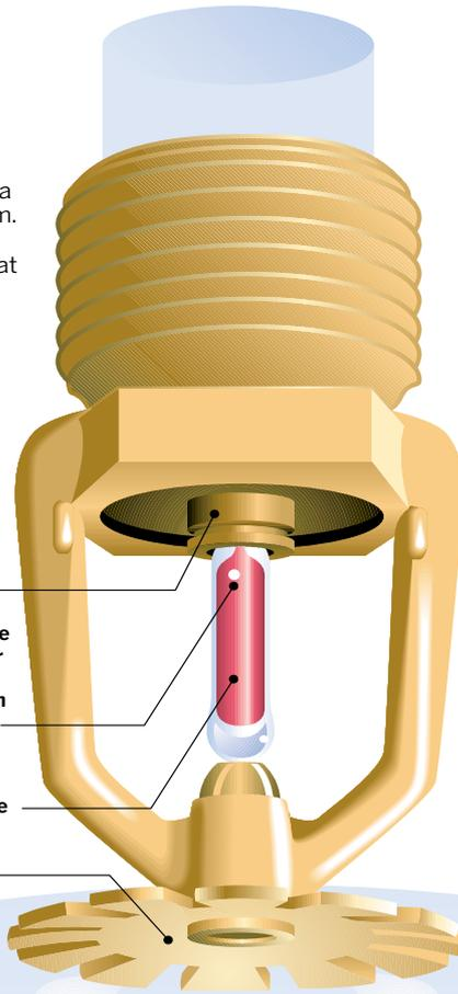
**2** This liquid is designed to expand and break the tube at a certain temperature. The most common are designed to break at 155 degrees. In the average sized room, a 5mm diameter ampule will usually break in about one to one and a half minutes from contact with a heat source. Ampules as thin as 1mm are manufactured for a faster response time.
