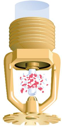
**3** The plug is forced out by the pressurized water behind it and deflected away by a beveled edge. The water sprays over the deflector plate which is designed to distribute it in an even pattern. Water will continue to flow until the main valve is shut off.
