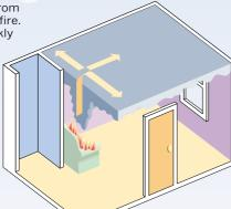
The current of hot air forces a curtain of deadly gases down the walls, making escape more difficult. In a few minutes the air will become so hot that the entire contents of the room will ignite spontaneously. This is known as flashover and usually occurs between 1,000 and 1,500 degrees.
