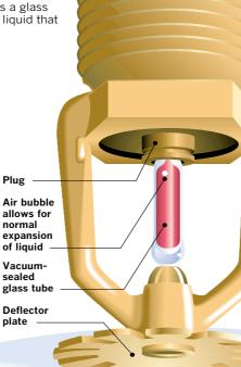
This liquid is designed to expand and break the tube at a certain temperature. The most common are designed to break at 155 degrees. In the average sized room, a 5mm diameter ampule will usually break in about one to one and a half minutes from contact with a heat source. Ampules as thin as 1mm are manufactured for a
