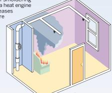
mechanism is heated to the required temperature, it trips and the water is released. The immediate cooling of the heat source usually prevents other sprinkler heads from activating. Often, one or two sprinkler heads are enough to control a fire.
